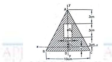
16. Support A has ball and socket connection. Roller support at B prevents motion in the -z direction. Corner C is tied to D by a rope. The triangle is weightless. Determine the unknown force components acting at A, B, and C. (14 marks)
