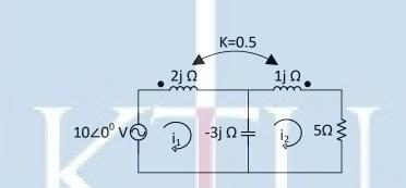
b) In figure,  $L_1=4H$ ,  $L_2=9H$ , coefficient of coupling K=0.5,  $i_1 = 5 \cos(50t-300)$  Amps,  $i_2 = 2\cos(50t-300)$  Amps. Write the KVL equations for V<sub>1</sub> and V<sub>2</sub>. Find their values at t=0 (4)
